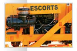
Proven, Powerful & Fuel efficient Kiloskar 4R 1040 TC water cooled diesel engine developing 76 hp
