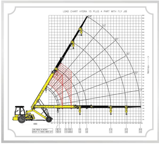
Rated loads are calculated for operation on levelled surface
